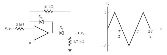
If op-amp and diodes are ideal, the output voltage waveform is
