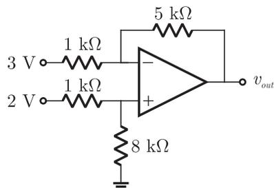
$$V_+ = \frac{8}{1+8}(3) = \frac{8}{3} \text{ k}\Omega$$
