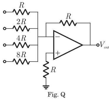
The input bits 0 and 1 are represented by 0 and 5 V respectively. The OP AMP is ideal, but all the resistance and the 5 v inputs have a tolerance of  $\pm 10\%$ . The specification (rounded to nearest multiple of 5%) for the tolerance of the DAC is
