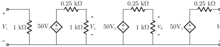
$$V_2 = \frac{1k}{1k + 0.25k} 50 V_1 = 40 V_1$$
