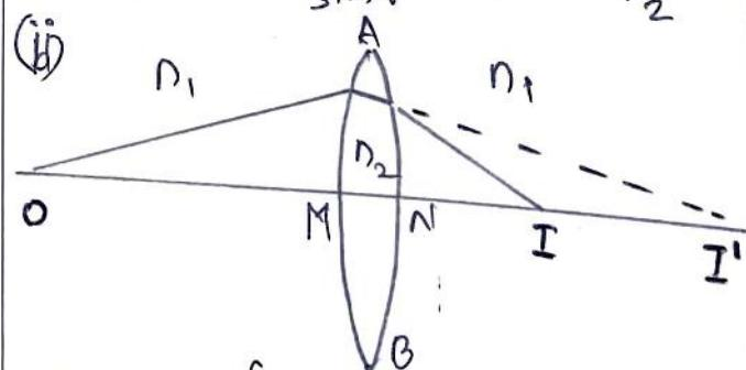
For surface AMB, image is formed at  $I'$ , with image distance, say  $v'$
