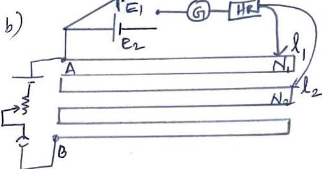
When the galvanometer is connected to  $E_1$ , we can apply Kirchhoff's rule for the loop  $A E_1 G N_1 A$  for the balancing length  $l_1$  as,
