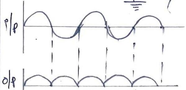
When an ac voltage is applied, during +ve half cycle,  $D_1$  is forward biased and  $D_2$  is reverse biased.
