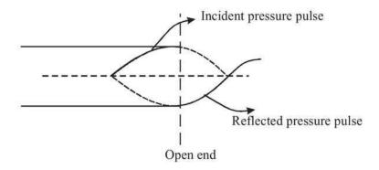
At open end pressure should not change pressure wave will get phase change as  $\pi$
