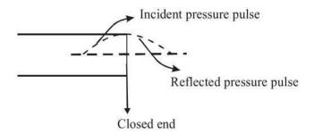
At enclosed end pressure wave will get reflected without phase change
