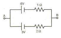
AB in volts is 36. [5] Total EMF = (6-3) V = 3 V  $i = \frac{3V}{3\Omega} = 1A$  $V_A - V_B = 3V + i \times 2 = 3V + 2V = 5V$ .
