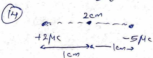
$$\begin{aligned} V &= V_1 + V_2 \\ &= \frac{1}{4\pi\epsilon_0} \frac{q_1}{r_1} + \frac{1}{4\pi\epsilon_0} \frac{q_2}{r_2} \\ &= 9 \times 10^9 \left[ \frac{2 \times 10^{-6}}{10^{-2}} + \frac{-5 \times 10^{-6}}{10^{-2}} \right] \\ &= 9 \times 10^9 \times 10^{-4} [2 - 5] \\ &= -27 \times 10^5 V \end{aligned}$$
