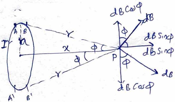
Magnetic field due to AB of length  $dl$  carries a current  $I$  at P,
