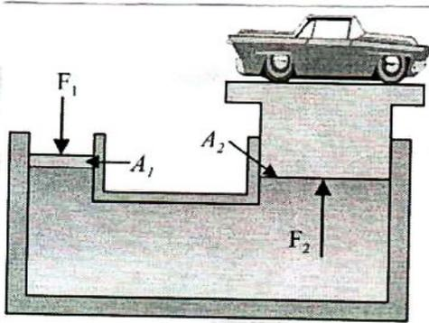
The pressure on smaller piston  $P = \frac{F_1}{A_1}$
