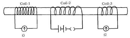
If the key connected to Coil-2 is plugged, in which of the other two coils more current is induced? Why?
