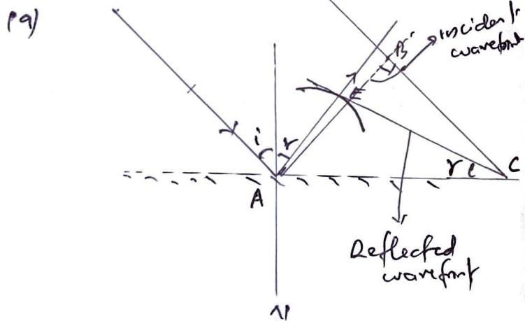
AB is an incident wavefront and EC is the reflected wavefront.
