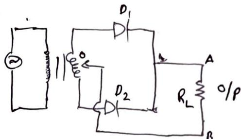
During +ve half cycle of ac input, D<sub>1</sub> is forward biased and D<sub>2</sub> is reverse biased and D<sub>1</sub> will conduct. Current flows from A to B.
